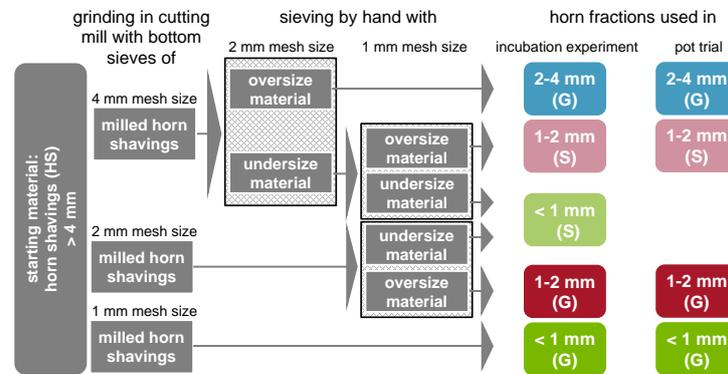
Fig. 1: Grinding and sieving procedure of horn shavings and resulting fractions (letter in brackets behind fractions indicates if upper particle size of the fraction corresponds to the mesh size of grinding (G) or sieving (S) procedure)
